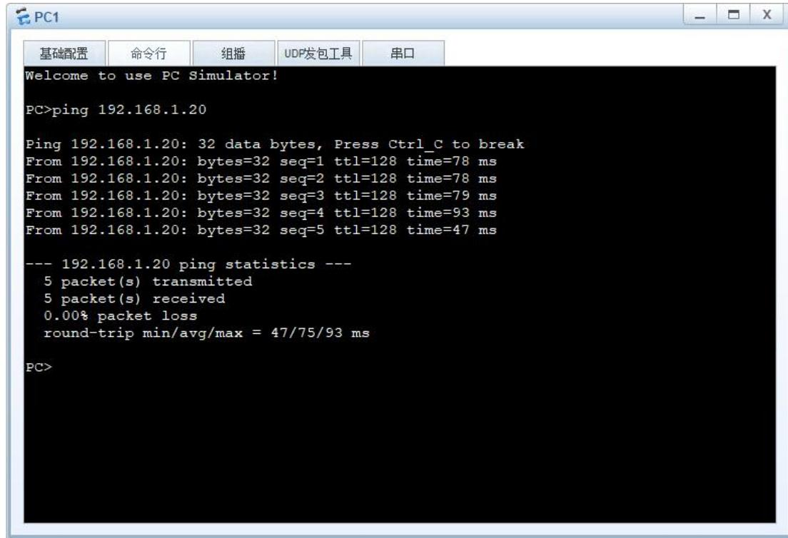
The screenshot shows a window titled "PC1" with tabs for "基础配置", "命令行", "组播", "UDP发包工具", and "串口". The "命令行" tab is selected, displaying the output of a ping command:
